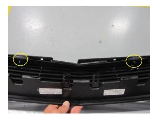
When properly installed, the billet grille will be secured to the factory surround at the four points show below in yellow.
