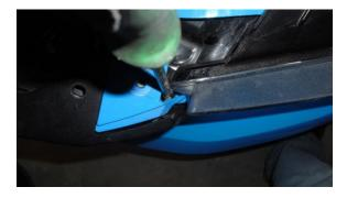
The below photo shows the mounting points of the grille to the front bumper cover. These must all be released to free the grille assembly from the vehicle.
